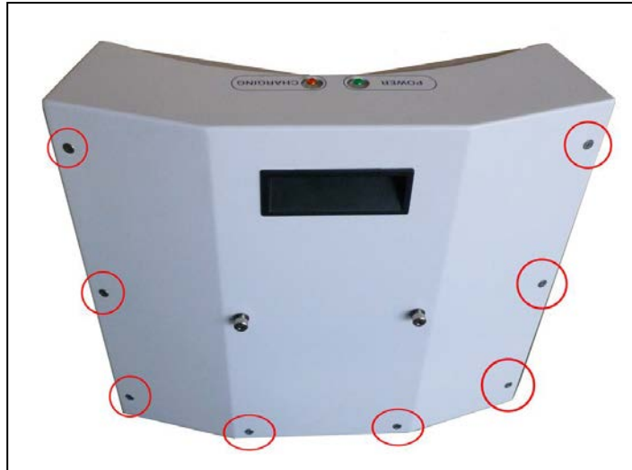
Figure 8-16 Docking Station Rear Cover Screws (8 of 10)
