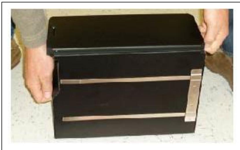
Figure 3-10 Correct Way to Lift the Battery
