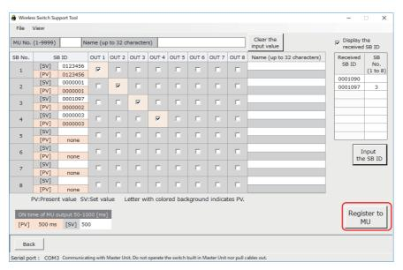
Slave buttons registration and output assignment settings, and one-shot output time of Master Unit are transferred to Master Unit.
