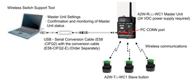
Note Install the driver for USB to serial conversion cable to computer before using USB to serial conversion cable with the conversion cable.
